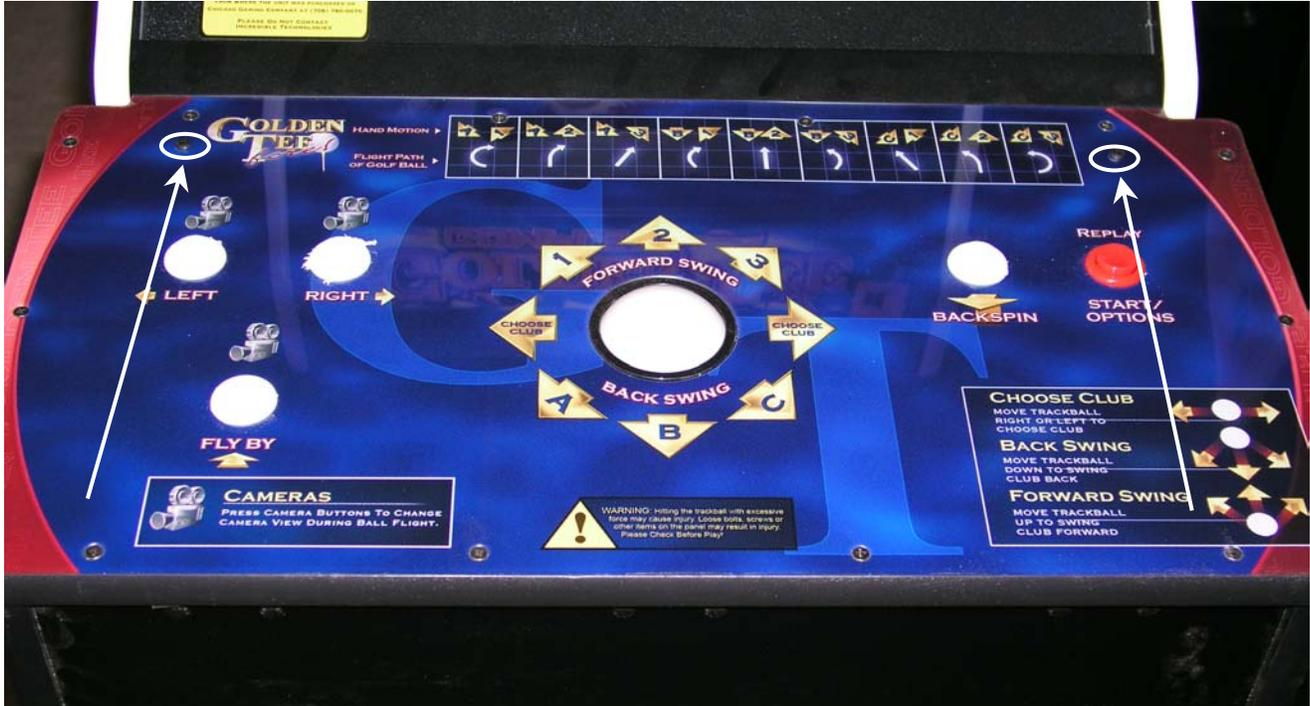
2. Once the screws are removed simply grasp the control panel, at the side nearest the screen, and gently pull upward. The panel is hinged at the front and will swing open. Once the panel is open, locate the latches on both sides and release them.
